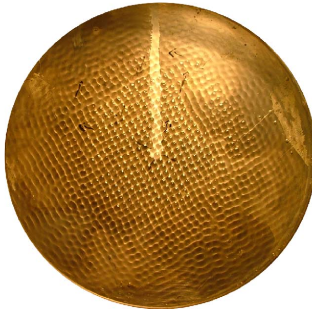
Fig. 2. Stationary waves at the fluid–air interface (top view of the plate). Driving acceleration W_d(0,0) : 13.8 \text{ m s}^{-2} .
